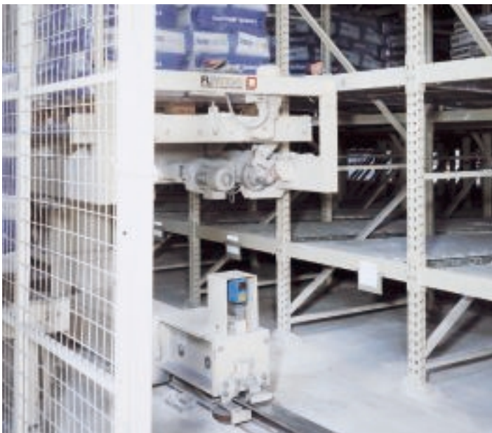
▲ Non-wearing, precise and flexible: A DME 3000 sensor used for positioning a rail-mounted rack-serving unit with millimetre precision; mechanical switches are no longer required, new docking points can be set quickly without any assembly requirements.
