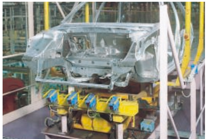
▲ A DME distance measuring device used to detect drill holes as part of inspection/quality control.
