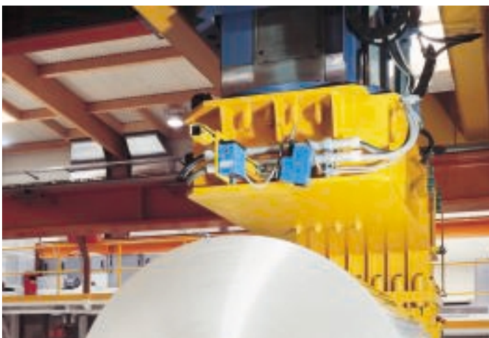
▲ DME process information: The weight of a coil can be determined from its diameter.
